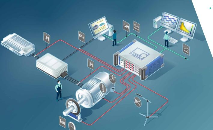
The eDrive solution from HBM covers the entire measurement chain: high-precision sensors, powerful instruments and intuitive software. Mechanical signals (e.g. torque) and electrical signals (current and voltage) are acquired simultaneously and help engineers to better understand the electrical drive and its losses faster and more accurately than ever before.
