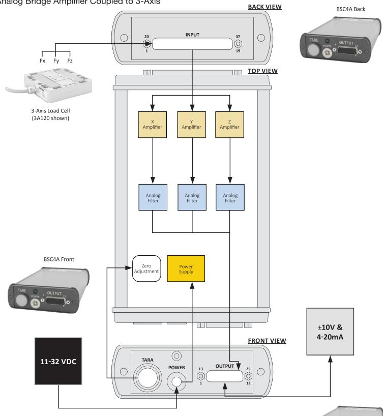
Note: This diagram is showing 3 channels to represent a 3-Axis system. The BCS4A has 4 channel capability.
