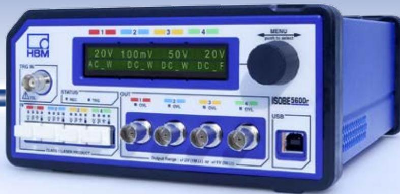
Receiver unit (with analog output or with memory)
