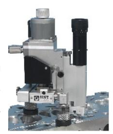
The heart of the system is the alignment-drilling unit, which is used to physically drill the hole and align the cutter with the center of the strain gage rosette by means of a cross reticule in the eyepiece. The system is also used, at the end of testing, to obtain the measurement of the hole diameter.
