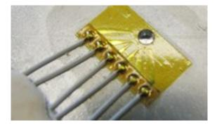
The hole-drilling method allows accurate experimental stress analyses at moderate costs. It consists in drilling a small hole (typically  $1.8-2.0\,$  mm) which changes the initial deformation allowing redistribution of residual stresses locked in a material.
